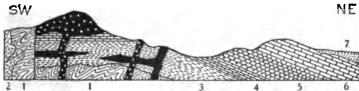
FIG. 738. — Section in the Thuringian Mountains of Germany, the region studied by Lehman, extending from the Inselberg (on the left) northeastward to Waltershausen. 1, 2, Urgebirge or Primary rocks (1, crystalline schist, 2, intrusive granite); 3-6, Flötzgebirge or Secondary rocks (3, Rothliegendes, tuffs and sandstones of Permian age; 4, Zechstein, Permian limestone; 5, Buntsandstein, Lower Triassic; 6, Muschelkalk, Middle Triassic. The Upper Triassic Keuper occurs in other sections). 7, Alluvium . Intruded porphyries in black, the younger with white dots. Note that the Secondary or Flötz of this region is older than that of the Saxon-Bohemian region, comprising Triassic and late Palæozoic (Permian). (Original.)
